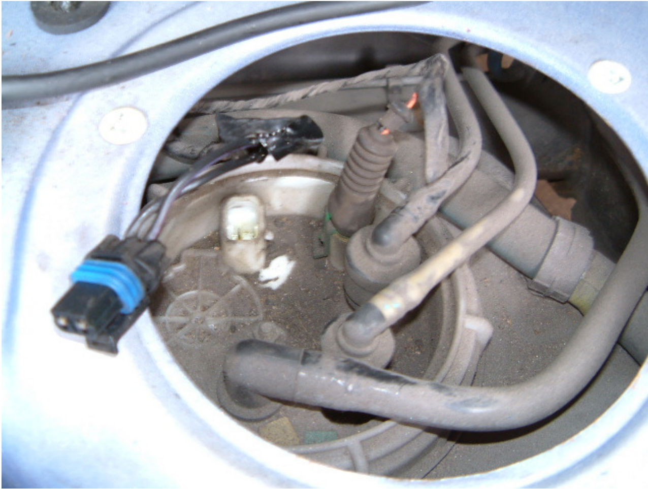
top of the fuel pump with the plug removed (Black -VE Black/Purple +VE)
