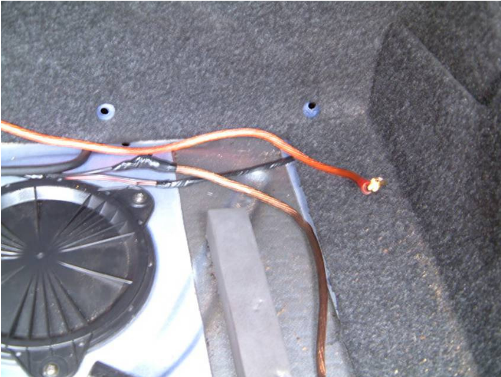
Earth wired up +VE in the boot just connected like this the voltage went up from 12.5 to 12.7
